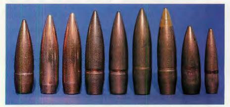
Projectile comparison (left to right): 7.62x51 147 gr. M-80 ball, Sierra .308 168 gr HPBT, Sierra 175 gr. HPBT, Soviet 152 gr. 7N1, Soviet 148 gr. LPS, Soviet 200 gr. Extra Match, Soviet 181 gr. Type D Heavy ball, 123 gr. 7.62x39, 52 gr. 5.45x39.
